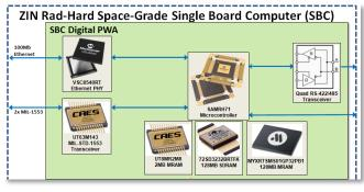
ZIN's Rad-Hard SBC was designed for Northrop Grumman's Habitation and Logistics Outpost (HALO)
